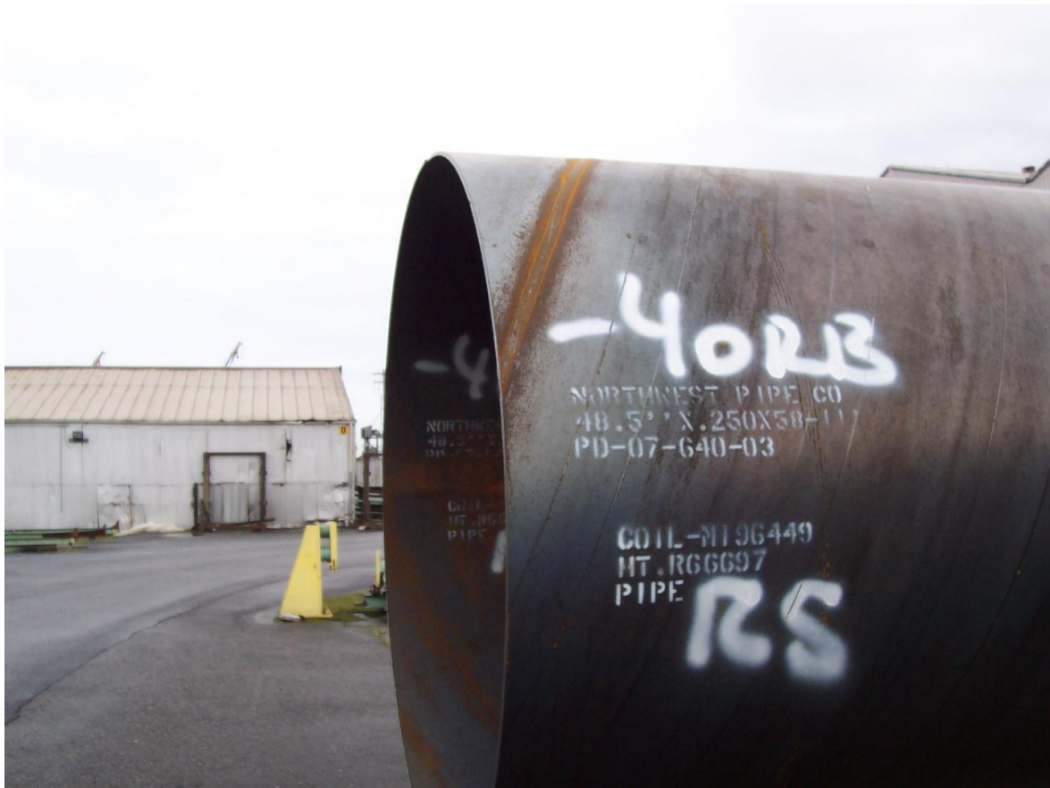
Figure 4 – Uncoated Welded Steel Pipe
