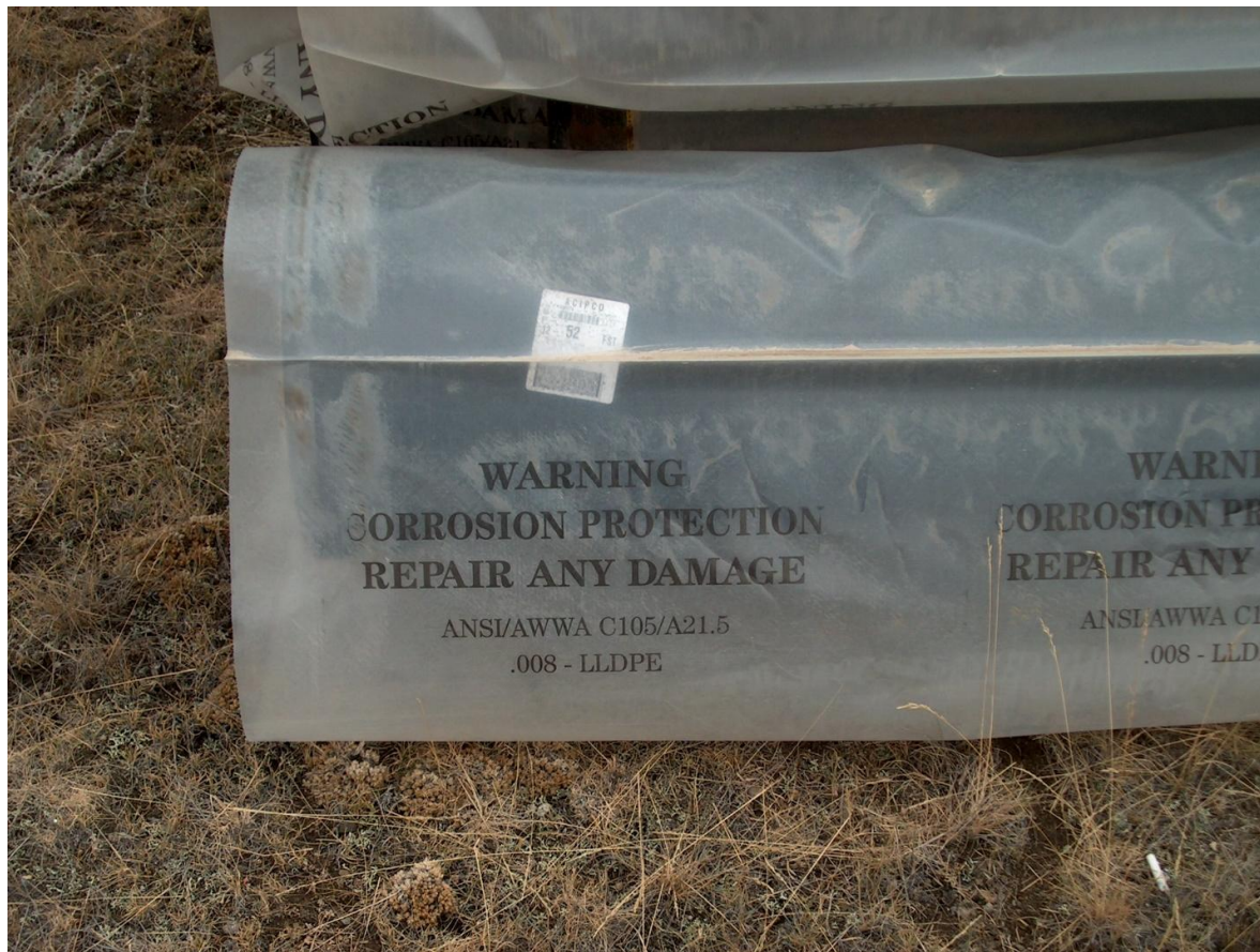
Figure 2 – Polyethylene encasement for ductile iron pipe
