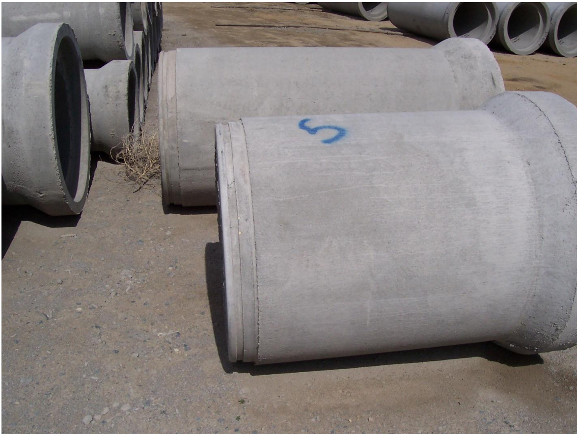
Figure 27 – RCP spigot end with groove for o-ring gasket
