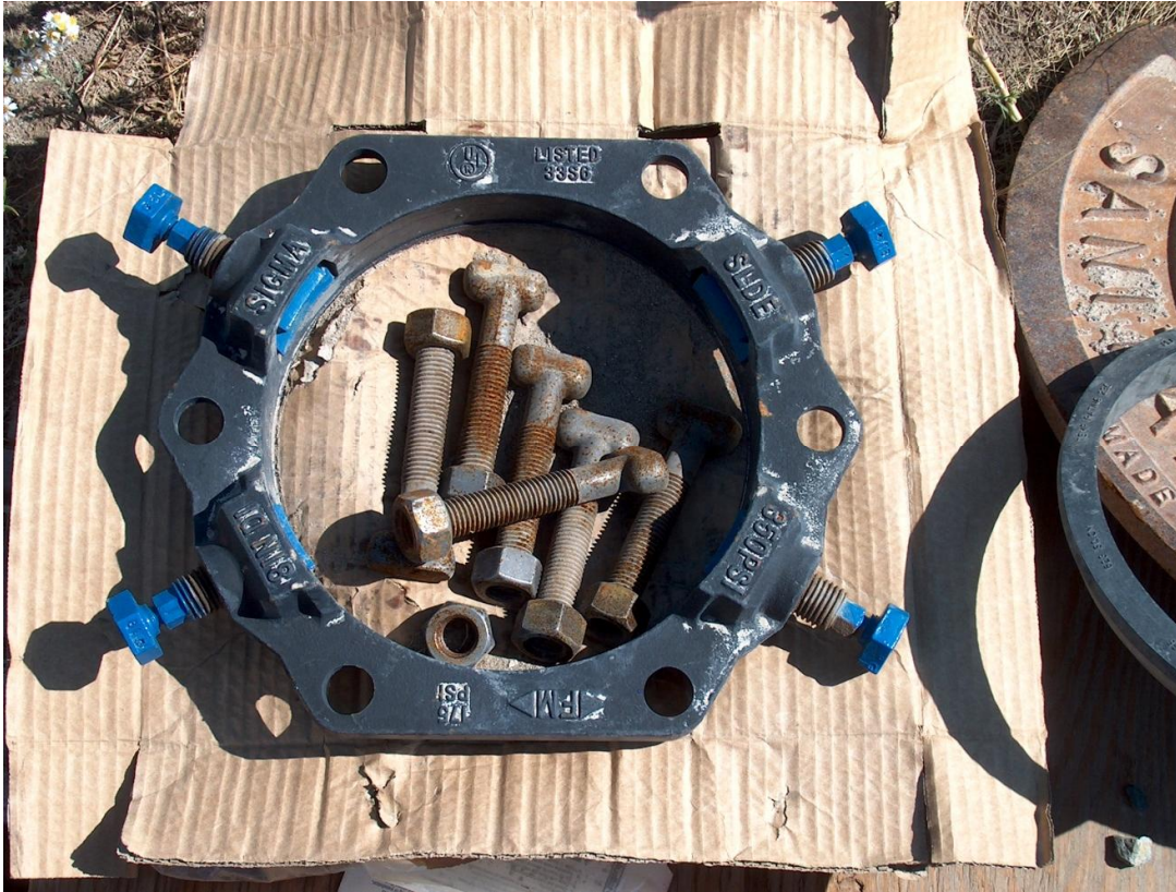
Figure 11 – Joint restraint for mechanical joint fitting
