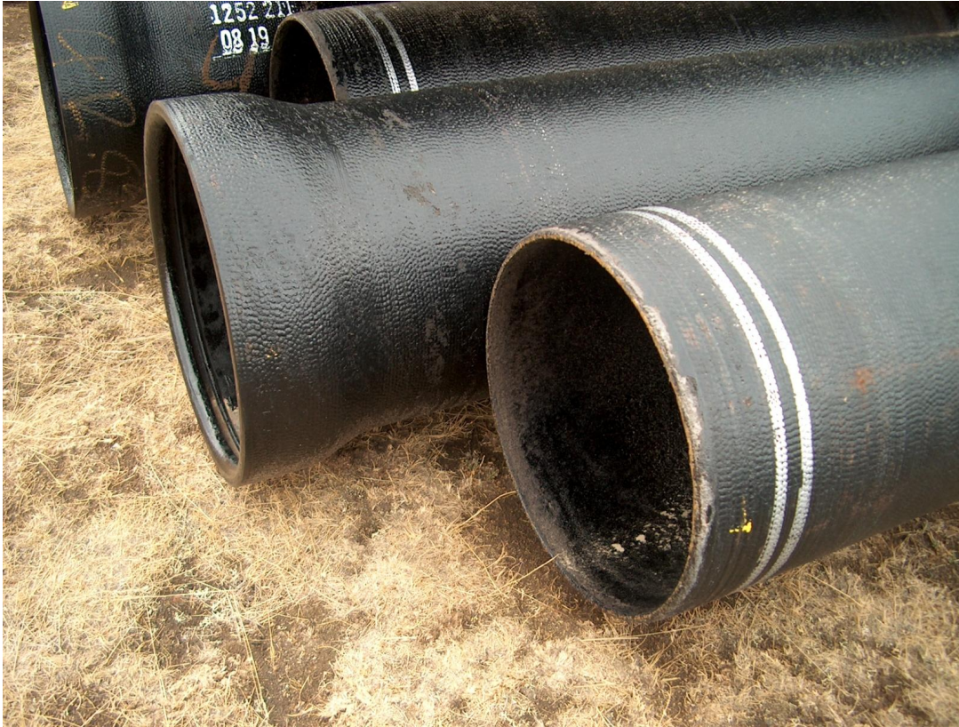
Figure 7 – Ductile Iron pipe with push-on joints
