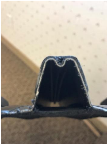
Figure 37 – Steel Reinforced Corrugated HDPE Cross-Section
