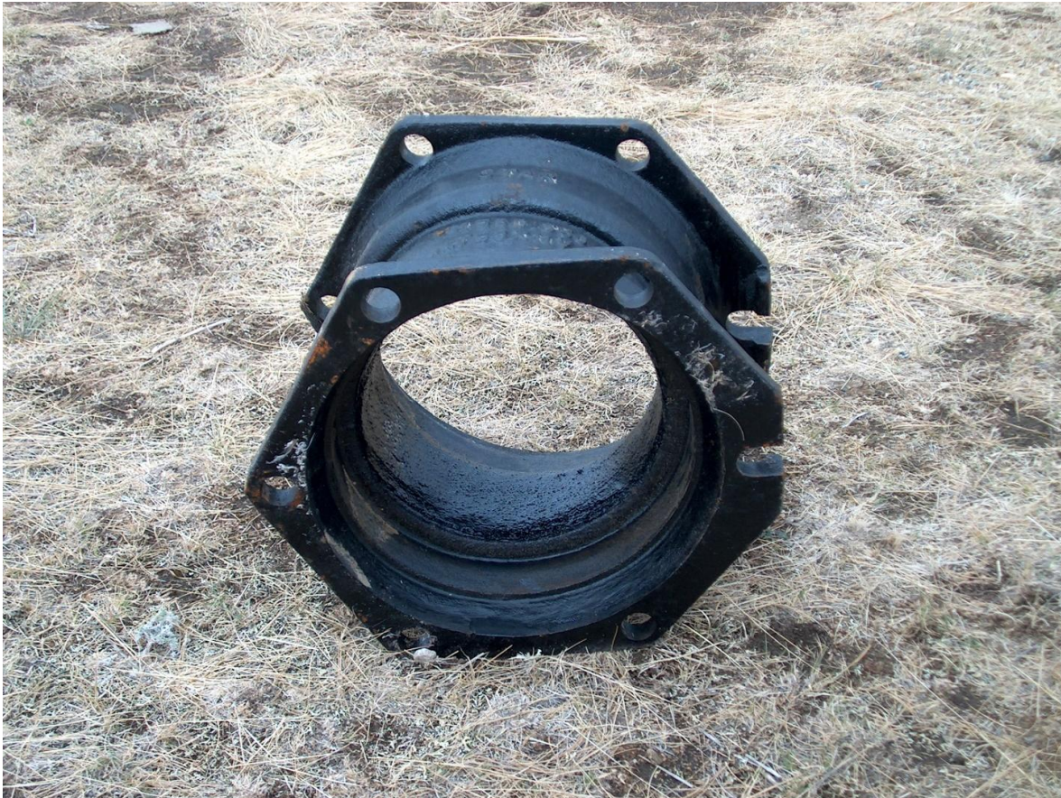
Figure 10 – Ductile Iron Pipe with Mechanical Joints
