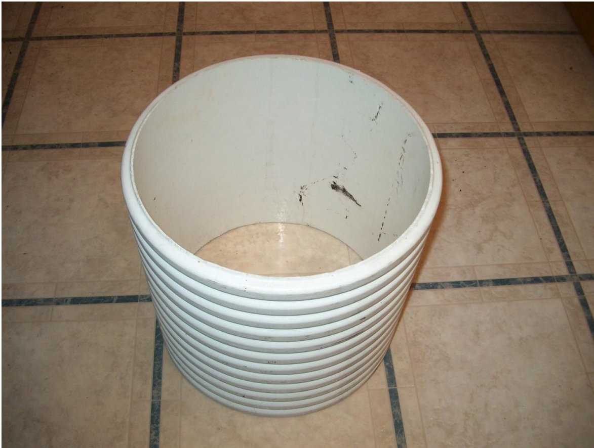
Figure 25 – Profile Wall PVC Pipe
