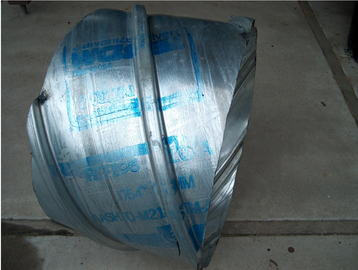
Figure 32 – Spiral Rib metal pipe
