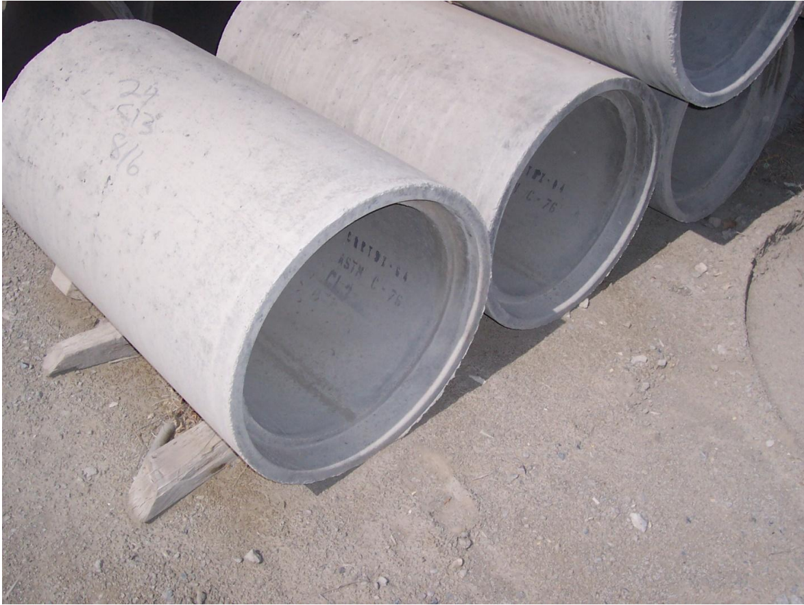
Figure 30 – RCP Groove End
