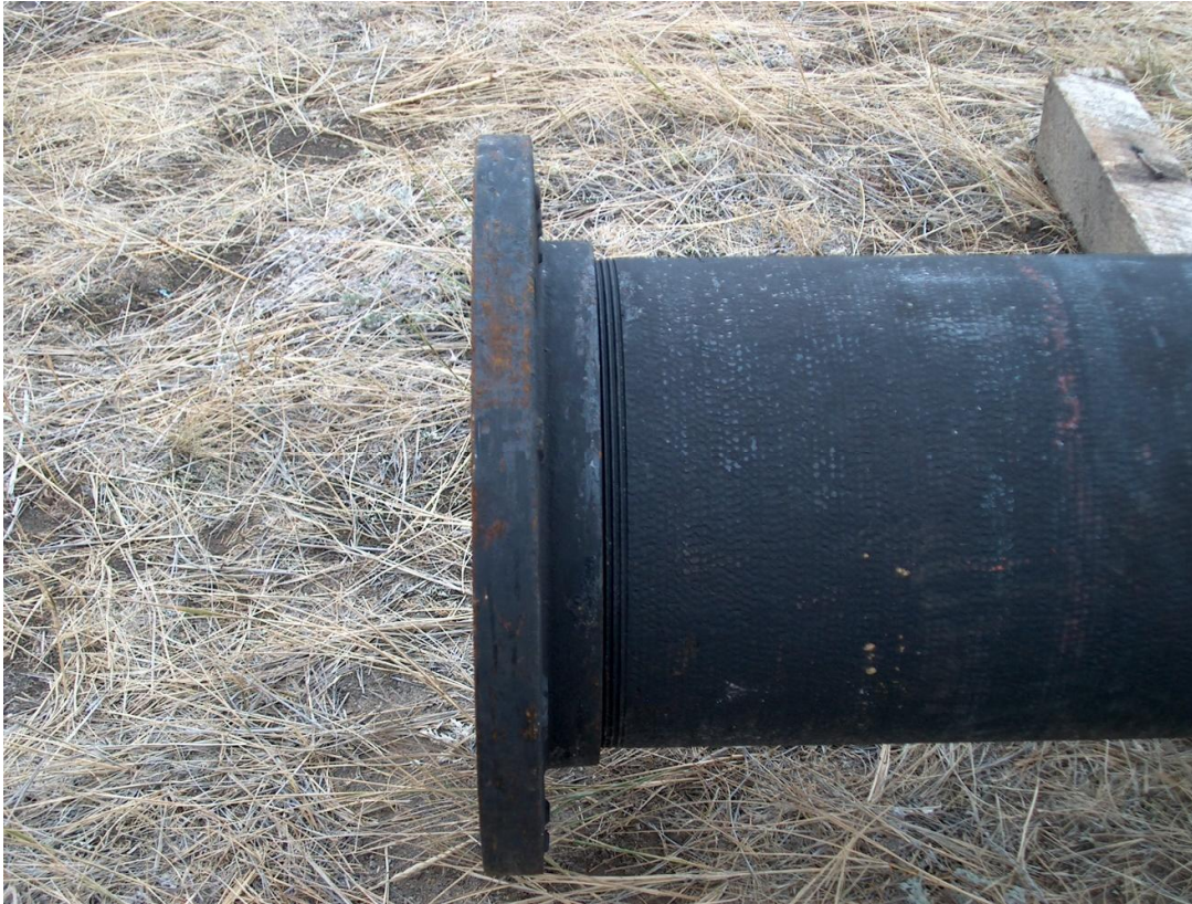
Figure 8 – Flanged Ductile Iron Pipe
