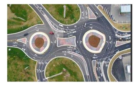
Careful attention should be paid to driveway connections where a traditional intersection is being converted to a roundabout. The driveway connections should not interfere with the pedestrian crossings or the yield zone.
