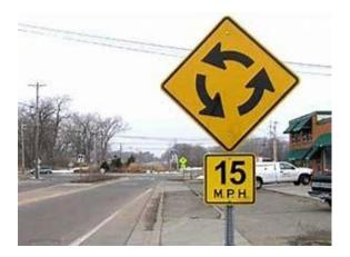
The roundabout ahead sign is an alternative to the circular intersection sign. At a minimum it is recommended that the roundabout ahead sign be used in place of the circular intersection sign at mini-roundabouts.
