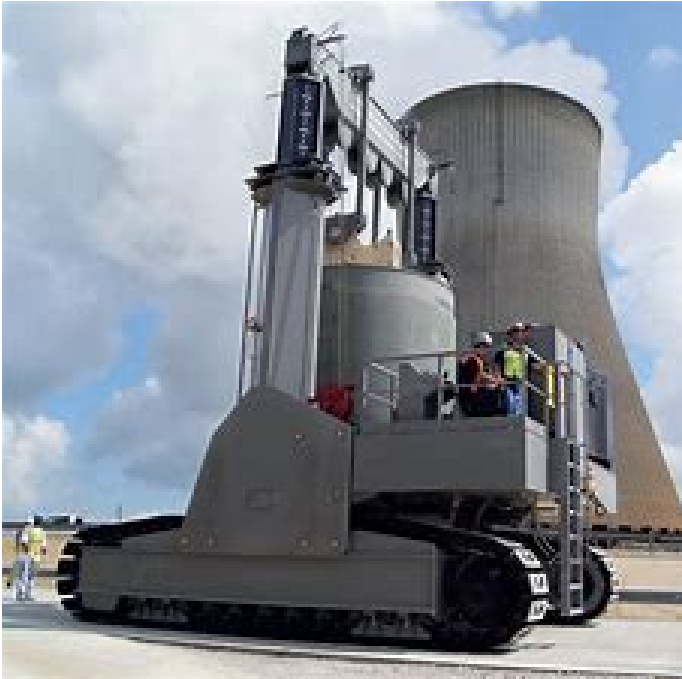
Figure 2-17: Vertical Cask Crawler 20
