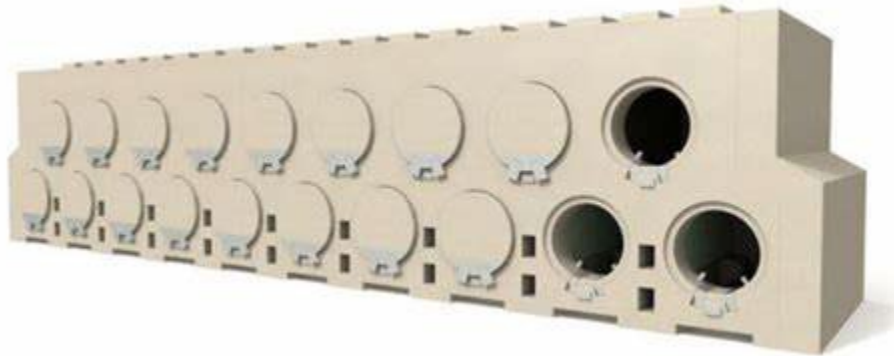
Figure 2-18: NUHOMS EOS Matrix DSS Design 21
