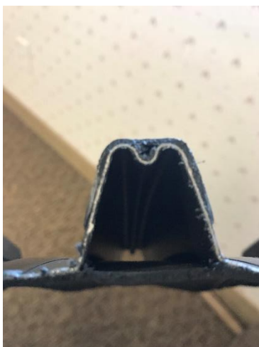
Figure 22 – Steel Reinforced Corrugated HDPE Cross-Section
