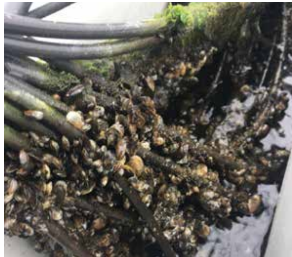
FIGURE 9.16 Biofouling on submerged connectors and cables
