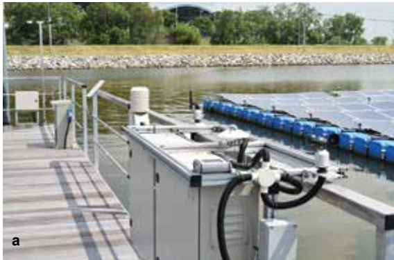
FIGURE 9.2 Meteorological station close to FPV system (a) and types of sensors: (b) wind speed sensor, (c) humidity sensor, (d) pyranometer, (e) Si-sensor, and (f) wind direction sensor
