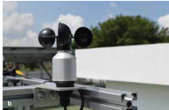
FIGURE 9.2 Meteorological station close to FPV system (a) and types of sensors: (b) wind speed sensor, (c) humidity sensor, (d) pyranometer, (e) Si-sensor, and (f) wind direction sensor
