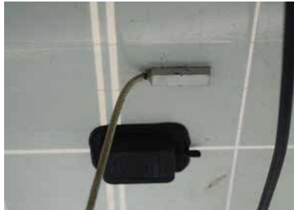
FIGURE 9.4 Examples of module temperature probes
