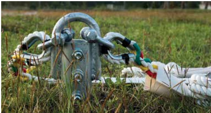
FIGURE 7.11 Land-based anchoring on the banks
